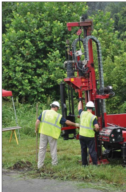
ABOVE AND BELOW: Kentucky Division of Waste Management staff watch a demonstration by Micah Group representatives on direct push/drill rig used to sample soil and groundwater. Photos by Micah Group
